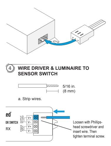
b. Wire Class 2 driver and LED luminaire to Sensor Switch. See **SYSTEM DIAGRAM.**
